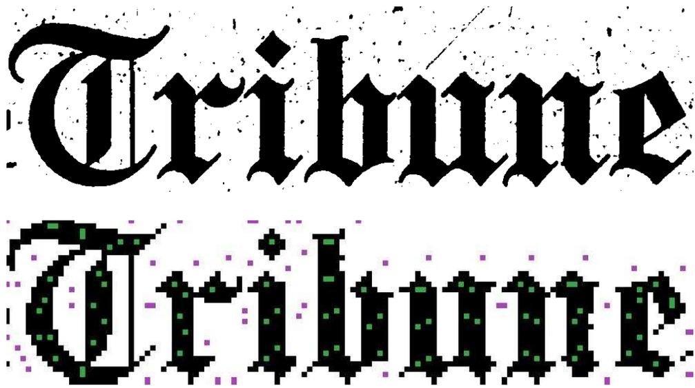
*Figure 7: Pattern and hit-miss Sel generated from it at 8x reduction.*
